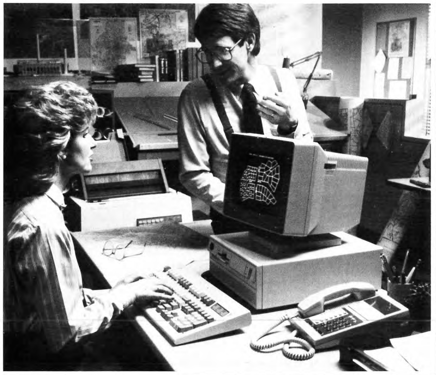
Fig. 1: IBM's 80286-based desktop model 50 and the new Personal System/2 monochrome display model 8053 being used to plot a subdivision. In the background, an IBM Quietwriter (R) III printer is ready to produce high-quality graphics.
